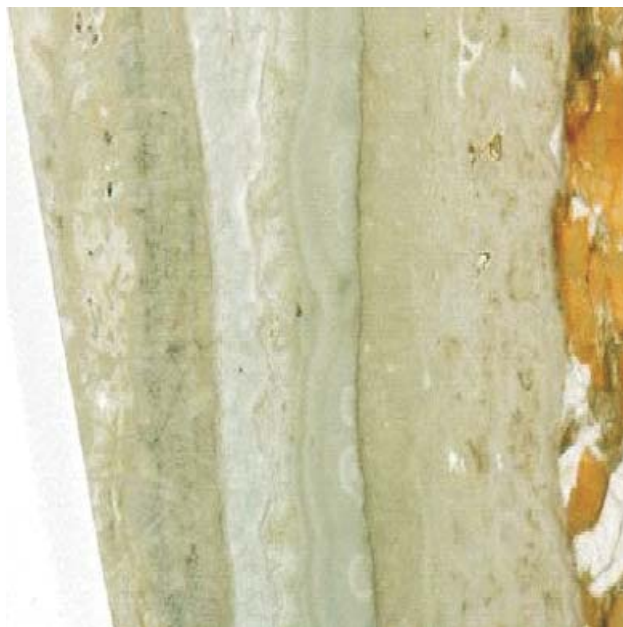
Figure 4. Alternating calcite-dolomite zones in the fissure infilling of the sample from 250.55 m in Borehole Üh-28
