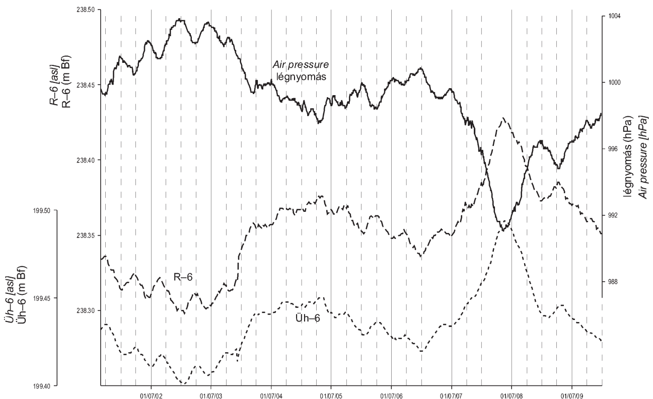
Figure 3. Connection between the water tables of observation wells Üh-6 and R-6 and the air pressure
